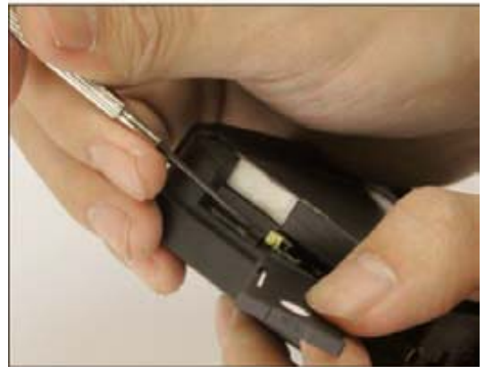
Removing the SIM holder.
